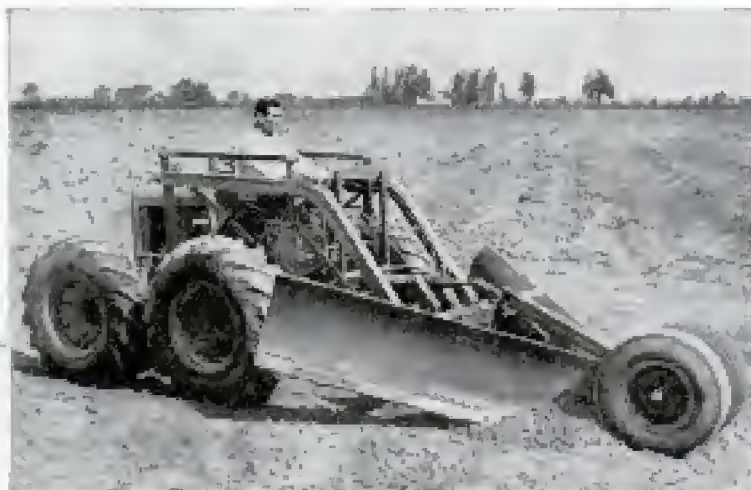
Another home-built machine is a hydraulic fork lift that will raise 1000 pounds to height of nine feet. Here it is used to move beehives to alfalfa field. Below, home-designed ditcher has two hydraulic controls to raise, lower and tip the blade
